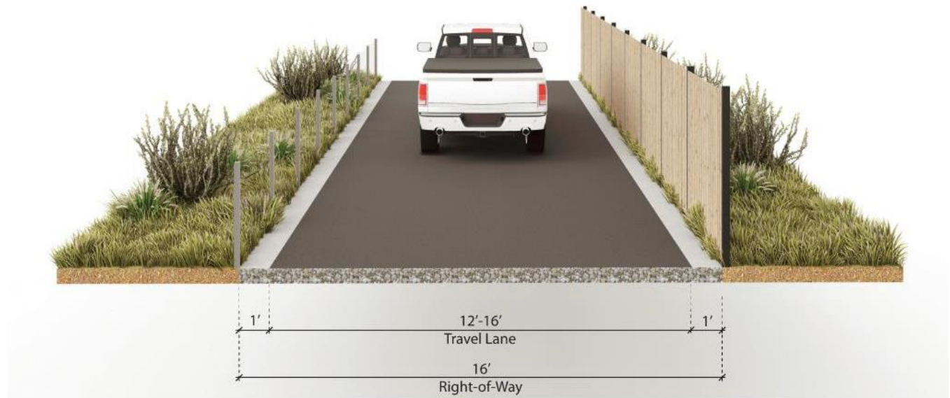
Figure 13: Cross-section for Alley
