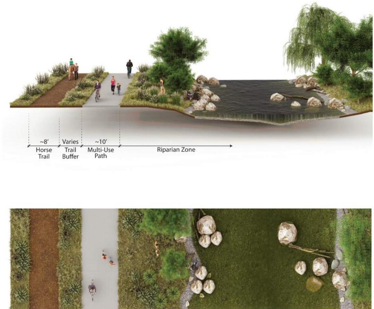
Figure 19: Cross-section for Umatilla River Multi-use Path and Horse Trail
