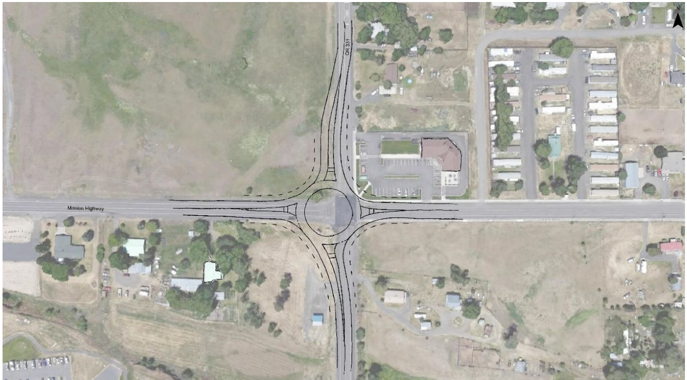
Figure A.6 Potential Roundabout Intersection Improvements
