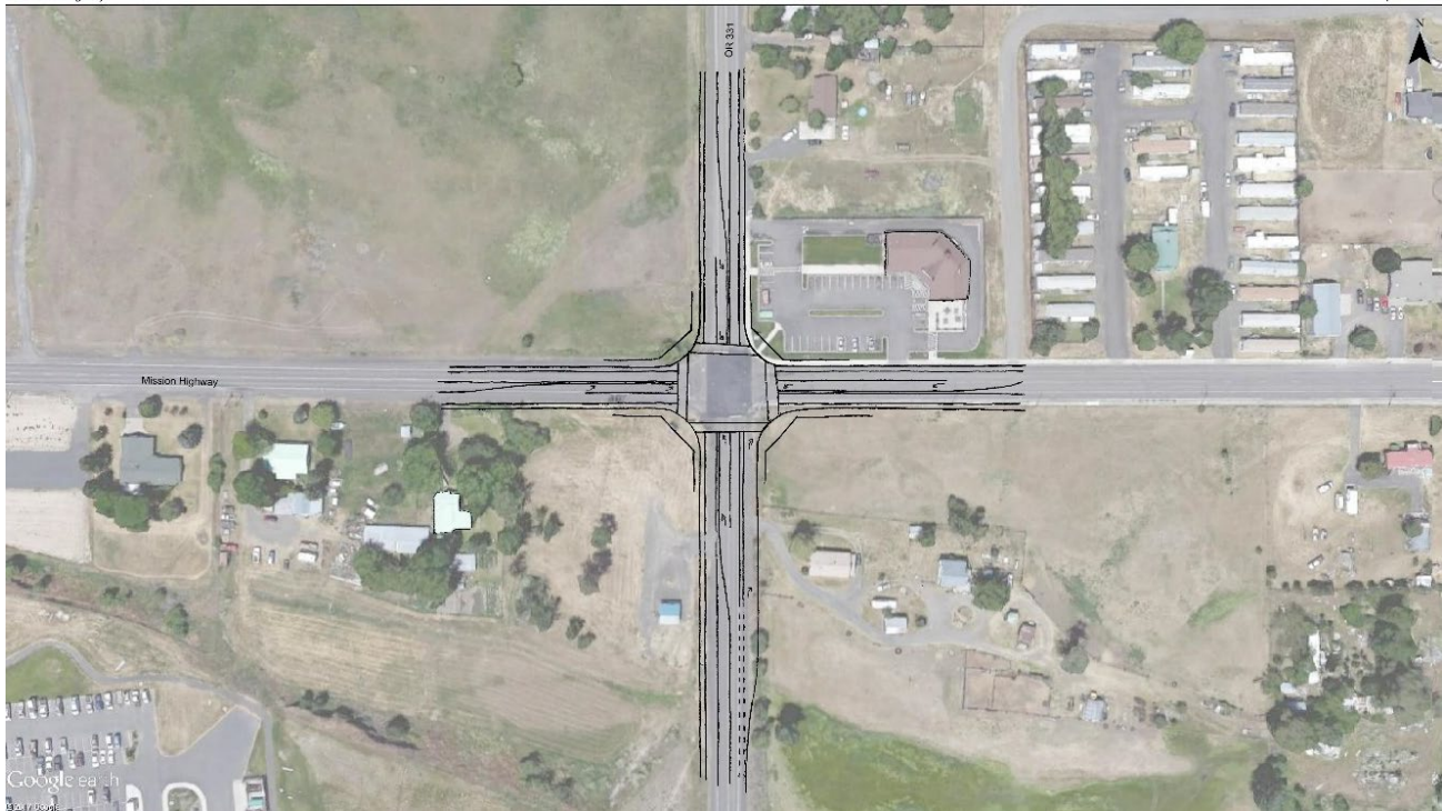
Figure A.5 Potential Signalized Intersection Widening Improvements
