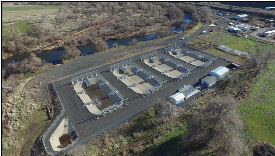
Aerial view the Pendleton acclimation facility showing the channel form that maintains flow to the water inlet structure without the need for gravel removal. The Imeques facility needs a similar type of channel at the inlet and outlet structures to eliminate the need for repeated in-river excavations after high flow events.
