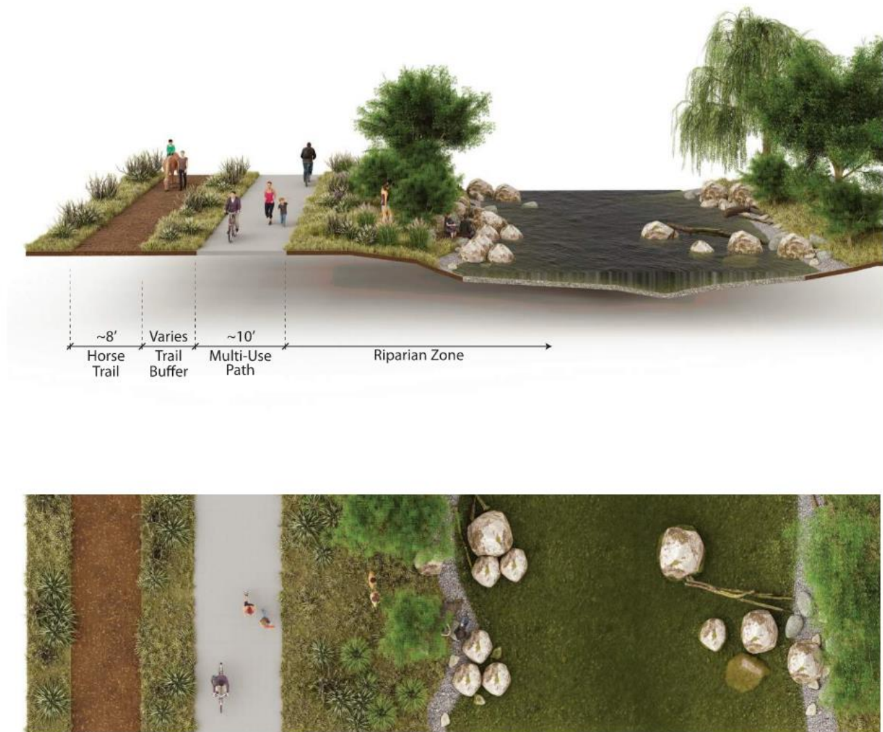
Figure 15: Cross-section for Umatilla River Multi-use Path and Horse Trail
