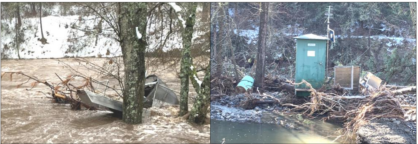
Climate events like the Feb 2020 flooding could potentially hamper CTUIR TAS status, through the disruption of information collection. Biomonitoring efforts like DNR Fisheries project effectiveness evaluation was temporarily disrupted by flood damage to rotatory traps (pictured left). This same flood event also damaged water quality monitoring equipment (pictured right) that is essential in measuring restoration efforts and impacts funding reporting.
