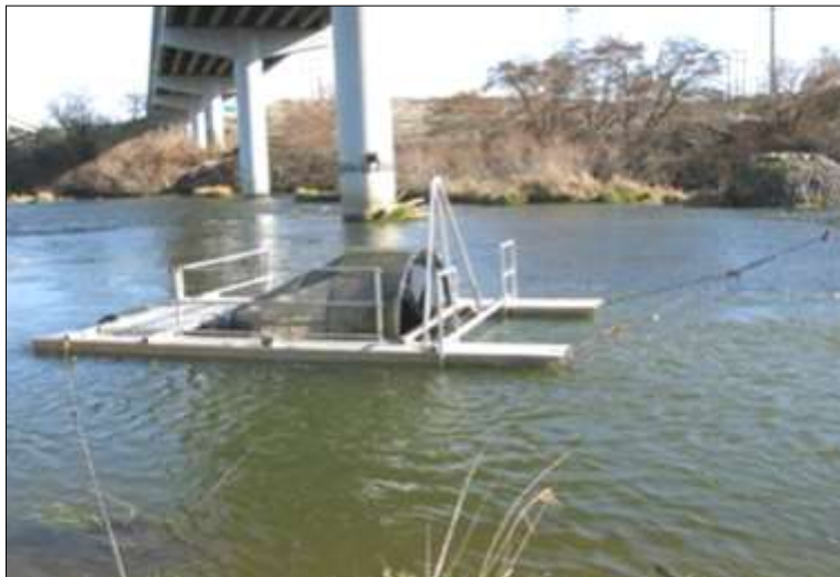
Rotary fish traps like this one on the Umatilla River temporarily trap fish to be counted before being released, as part of CTUIR project monitoring and effectiveness evaluation. This kind of data collection also informs harvest regulation and management actions.
