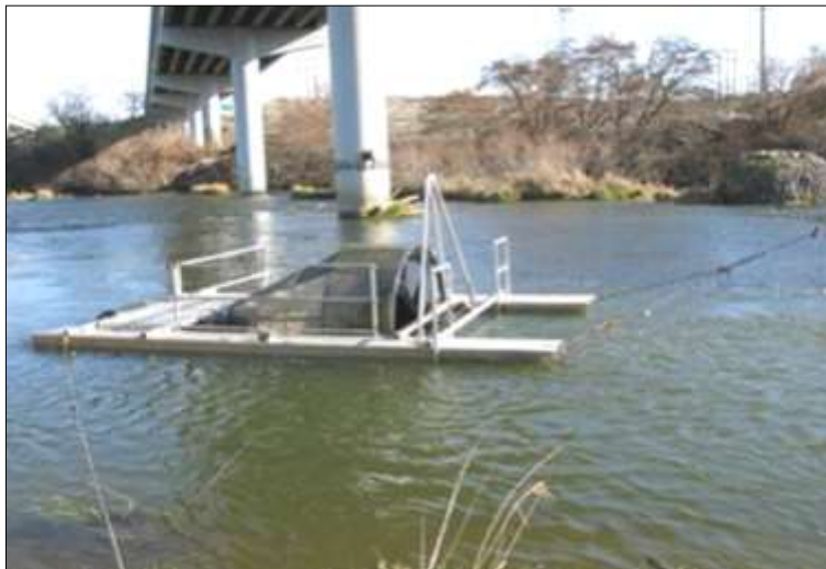
Rotary fish traps like this one on the Umatilla River temporarily trap fish to be counted before being released, as part of CTUIR project monitoring and effectiveness evaluation. This kind of data collection also informs harvest regulation and management actions.
