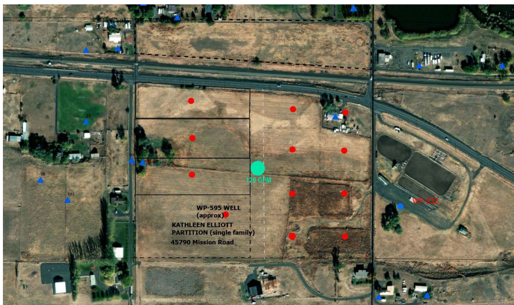
Fig. 1 UM-70 showing proposed location of WP-595 development well, eleven additional wells (red circles), modeled community well (green circle), Mustang well (blue circle) and existing wells (blue triangles).
